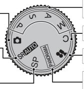
**P, S, A, M**: Select for full control over camera settings, including aperture (**M** and **A**) and/or shutter speed (**M** and **S**) (pg. 27).
